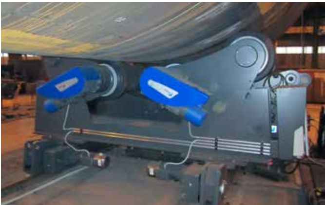
PEMA A rollerbeds ascertain even weight distribution on the work-piece.
