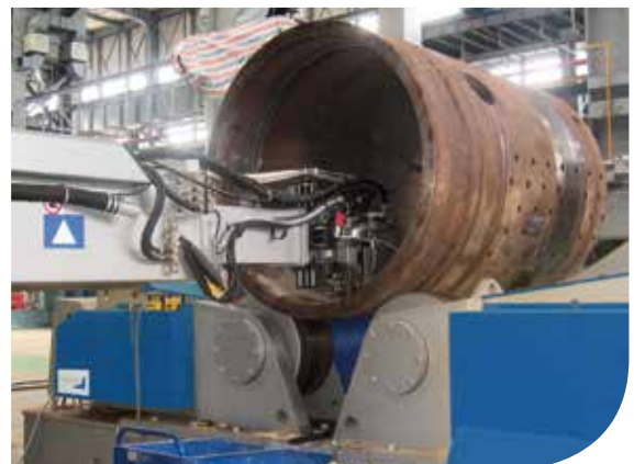
Welding carried out by means of a column & boom and a set of heavy PEMA N rollerbeds
