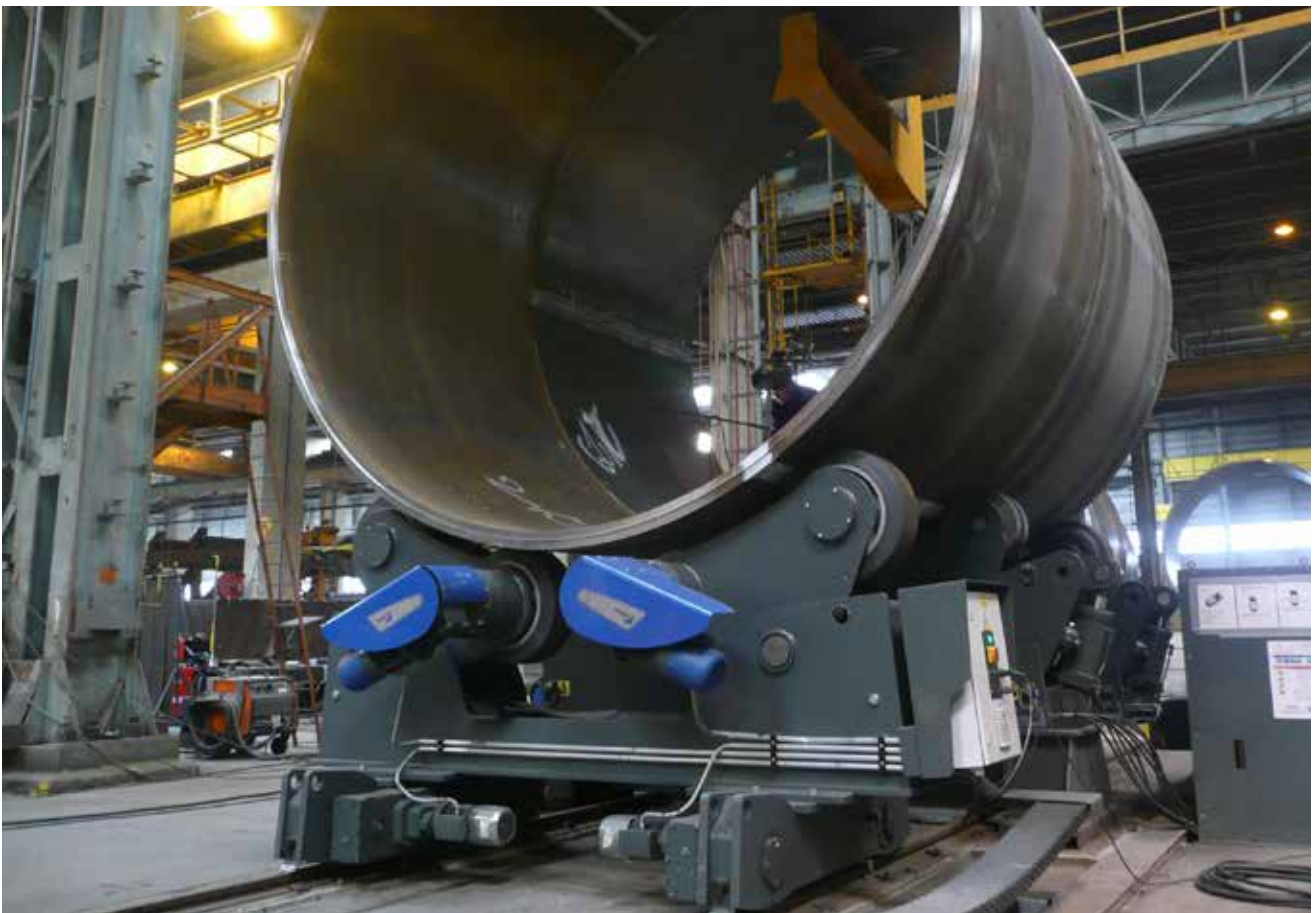
PEMA rollerbeds can be equipped with rail cars to enhance the efficiency of production material flows.
