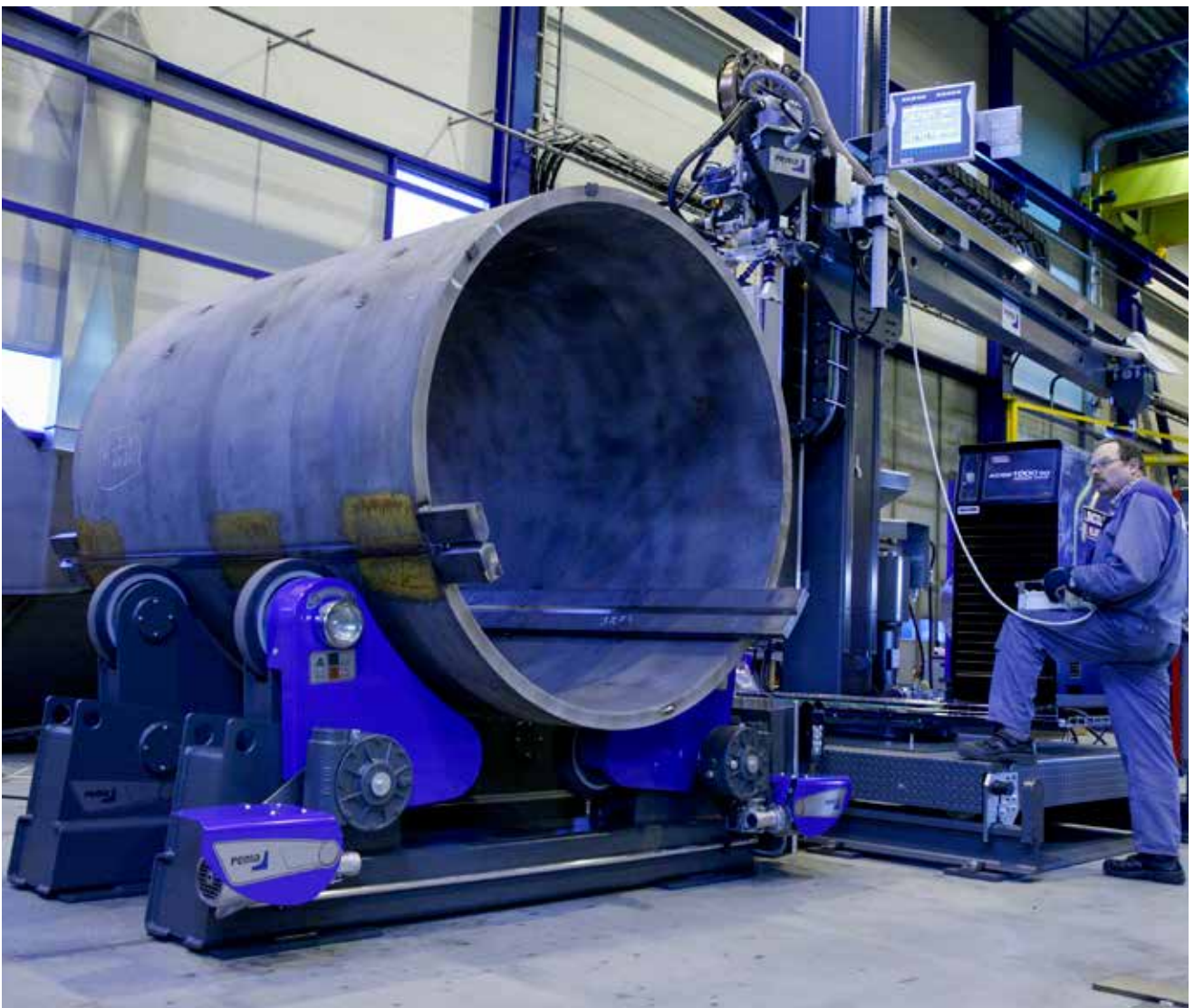
PEMA rollerbeds with PEMA column & booms complement even the most demanding hard automation solutions.
