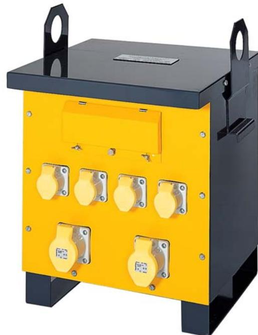
The outlet sockets on this transformer are manufactured by Defender and 'Walther' and are approved to BS EN 60309. The MCB's are installed; 1 x 20A in series with 2 x 16A outlets, 1 x 20A in series with the other 2 x 16A outlets, 1 x 32A on each of the 32A outlets and 1 x 50A on the input.
