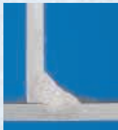
With start-up program - no fusion defects
