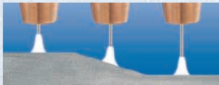
Constant arc length, despite changes in the stick-out
